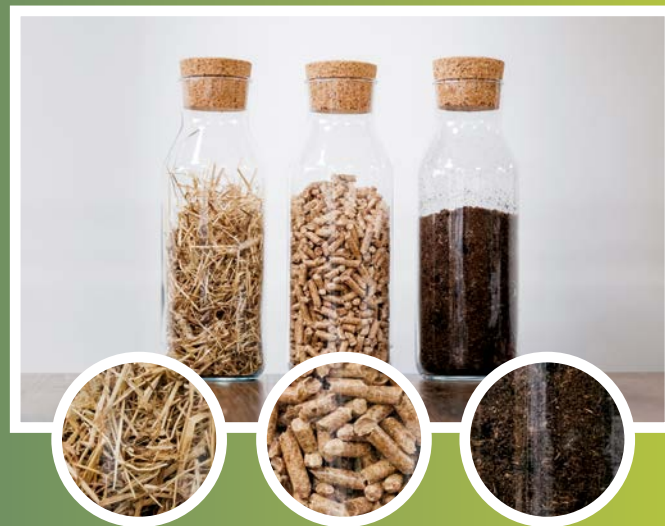
Figure 2: Straw, wood pellets and compost – just three of the biogenic material feedstocks that the team at Wild Hydrogen have been investigating for hydrogen generation
