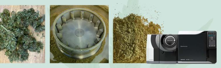
Figure 8: Cannabis flowers before grinding and after cryogenic grinding in a ball mill (total of 4 min for 20 g sample) or the ZM 300 (10 min for 500 g sample)
