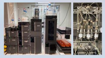
Figure 4: Shimadzu's ultrafast preparative LC system used at Exscientia, showing the complete setup (left) and the fraction-trapping capability (right) that was vital for avoiding lengthy dry-down procedures
