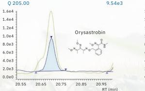
Figure 4: Comparison of waveform processing results by Peakintelligence for GCMS and conventional waveform processing
