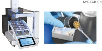
Figure 3: The EDGE from CEM (left). Filling the homogenized sample into the Q-Cup before extraction (right).
