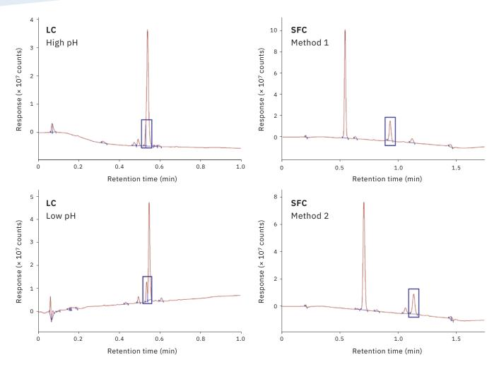
Figure 3: Example of exploratory purification work carried out at Exscientia on an impure sample, showing two LC separations at different pH (left) and two SFC separations using different methods (right). Both SFC methods easily separate a significant impurity that is only partially resolved or completely unresolved using LC.
