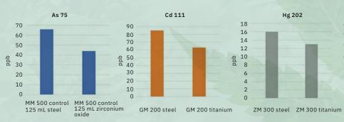
Figure 12: Effects of the correct grinding tool on analysis results. The abrasion from steel tools leads to higher heavy metal values, which distorts the analysis. This can be avoided by using zirconium oxide or titanium tools.
