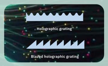
Figure 3: Groove shape of diffraction grating
