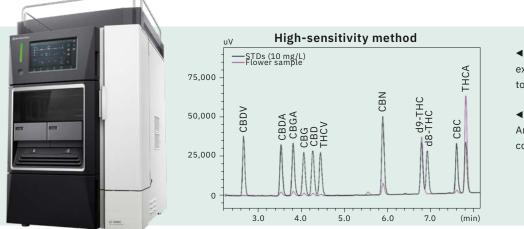
Figure 4: Chromatogram of an extract from hemp flowers compared to a standard solution
