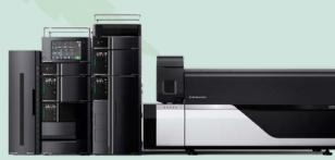
Figure 10: LCMS-8060NX for detecting pesticides and mycotoxins
