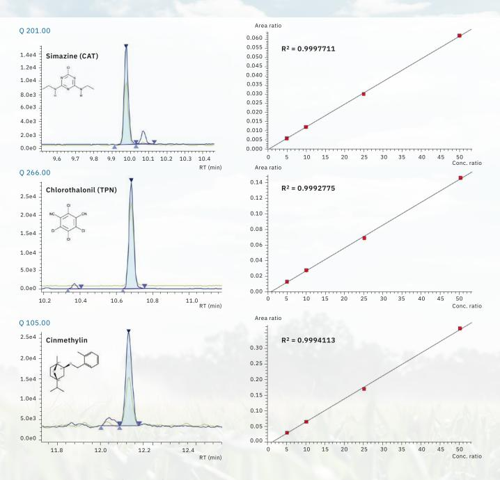
Figure 3: SIM chromatograms (0.005 mg/L) and calibration curves of agricultural chemicals in water
